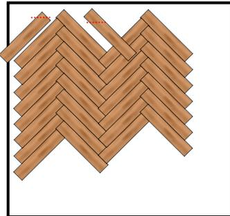
Planks or tiles will need to be cut to allow finishing up against a static object such as a wall, skirting board or Radiator Pipe, when cut make sure that the board fits free of the static object.
