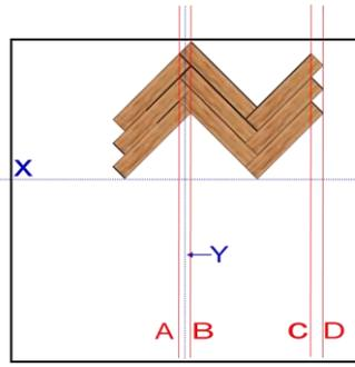
The A and B lines pass through the top points of the left and right planks, using a chalk line they are equally spaced from the Y axis line. This will help maintain your pattern.
