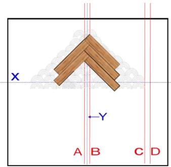
The herringbone planks can then be laid into the adhesive, remember to observe any direction arrows printed on the underside of the plank or tile.
