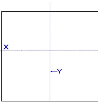
A herringbone design should typically be started from a central axis, using a chalk line or straight edge to mark the centre of your room create the 'x' line, then a second line needs to intersect this line at 90° to create the 'y' line. Setting this axis up is crucial and its good practice to check all angles and measurements are correct at this stage before any planks are laid.
